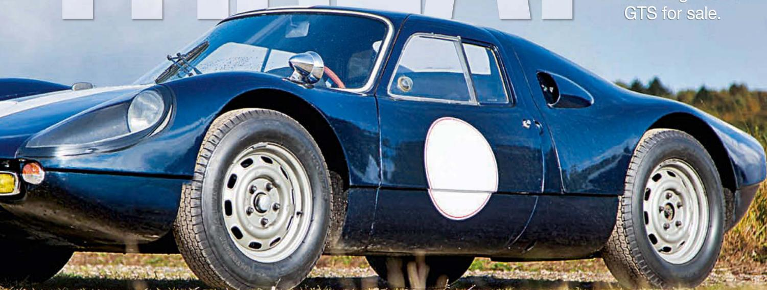
The body comprised 50 separate GRP parts, and in combination with the frame chassis and engine it would weigh just 740kg in total, but with everything bolted to the frame it actually boasted a high level of torsional stiffness.
